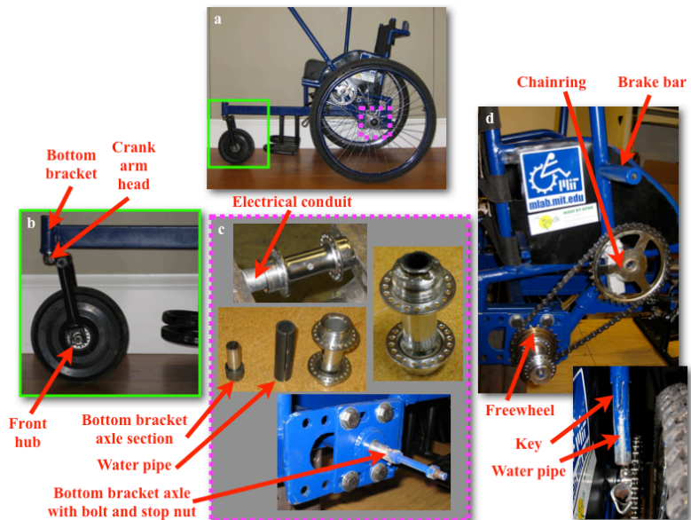
Figure 2. LFC bicycle part construction. a) All moving parts on the LFC are made from bicycle components. b) The front caster assembly. c) The rear hub and axle assembly, with hub inserts made from electrical conduit and water pipe. d) Lever coupling to drivetrain made from water pipe.
