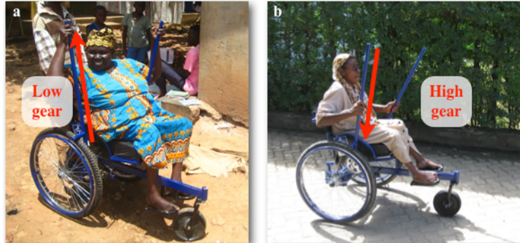
Figure 1. Moving hand position on the LFC levers changes mechanical advantage. a) Placing hands high on the levers generates high torque and an effective low gear. b) Placing hands low on the levers creates high angular velocity in the drivetrain and an effective high gear.
